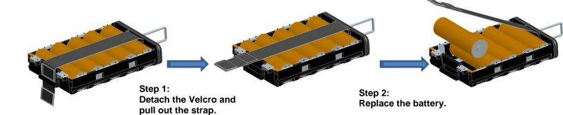
WARNING: RE-USING OLD BATTERIES OR MIXING OLD AND NEW BATTERIES IN THE IN-CAR UNIT MAY DAMAGE THE ELECTRONICS.
