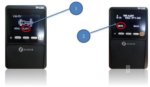
Wake up – unit will produce "two tones (High-low)", this shows that In-Car unit is awake and operational.
